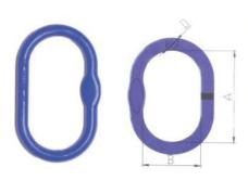
Green painted other colour is available as per request. Working load limit permanently shown on the body. Max proof load is 2.5 times of the working load limited. Min.Breaking strength is 4 times of the W.L.L.
